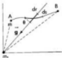
$$\Delta E_p = Gmm_1 \left( -\frac{1}{r} \right)_{r_A}^{r_B} = - \left( G \frac{mm_1}{r_B} - G \frac{mm_1}{r_A} \right)$$
